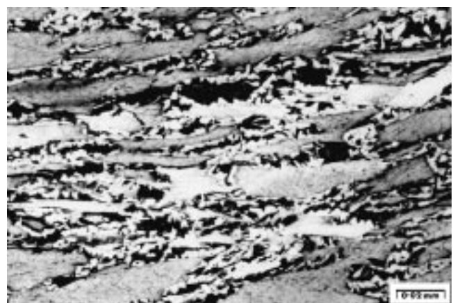
Fig. 11 Microstructure of steel A warm rolled to 48% at 780 °C followed by oil quench shows the presence of epitaxial ferrite
